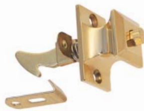
1283-PB Base of knob: 1 3/16" X 1 5/16" Projection: 13/16" Solid brass with steel parts Push catch with knob For door thickness 1/4" to 3/4"
