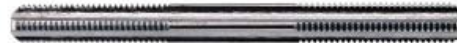
8839-20 Straight spindle 9/32" (7mm) wide 8777-20 Straight spindle 5/16" (8 mm) wide Length: 4", thread: 3/8 - 20, zinc plated steel Available in two widths
