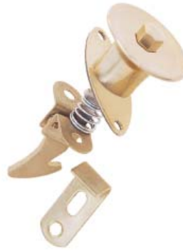
1290-PB Knob 1 1/8" dia. , 3/4" projection Oval base: 1 1/2" X 11/16" Stamped brass with steel parts Push catch with knob For door thickness 1/4" to 7/8"
