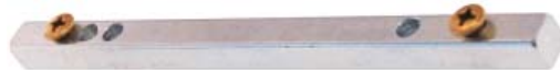
8774 Plain straight spindle Length: 4 1/2", width: 9/32" (7mm), zinc plated steel Door thickness range: from 1 3/8" to 2 1/2" Plain unthreaded spindle with 5 threaded holes for screws Comes with two 10-24 X 3/8" set screws (shown below)
