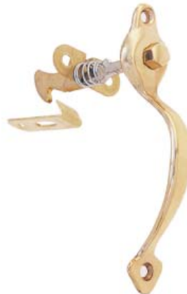
1284 -PB Handle: 3 3/8" high , 3/4" wide Projection: 3/4" Solid brass with steel parts Push catch with Handle For door thickness 1/2" to 1"
